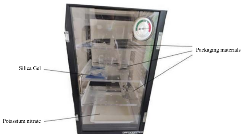
Plate 4: Accelerated shelf life testing set-up according to ASTM 19
